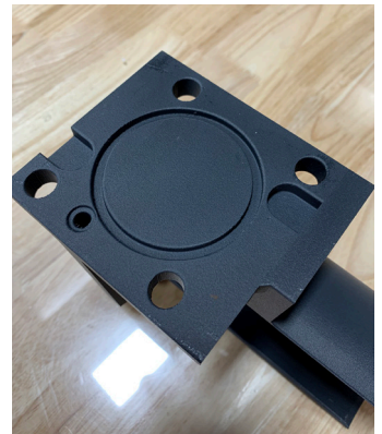
The mounting flange of the part catcher shows the surface finish achievable with FDM Nylon-CF10 material.
